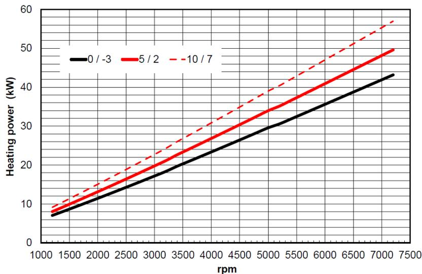
ELECTRIC POWER (400 V 3/N/PE). Heating 40/45 °C. Brine 0/-3, 5/2 y 10/7.
