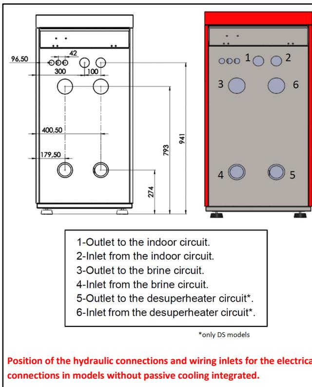
Position of the hydraulic connections and wiring inlets for the electrical connections in models without passive cooling integrated.
