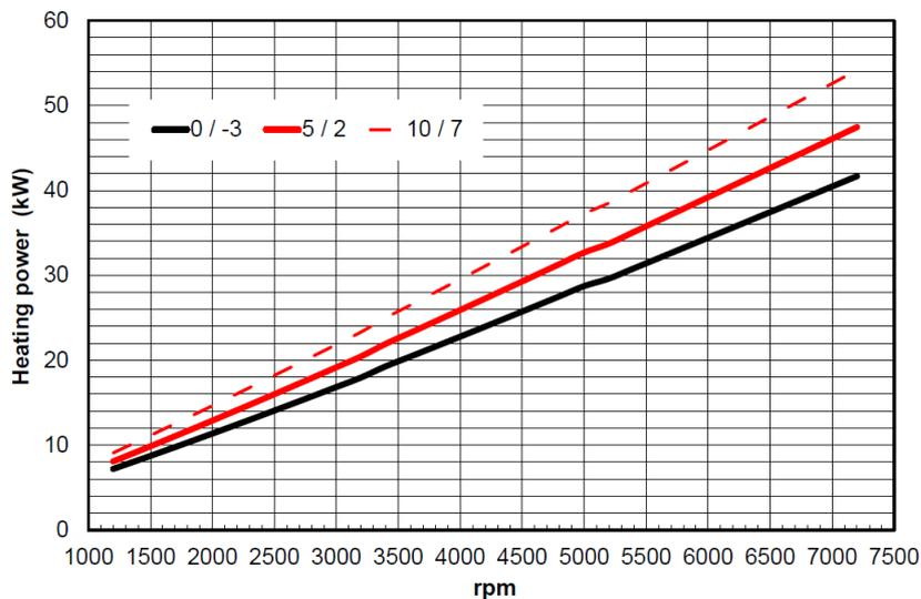
ELECTRIC POWER (400 V 3/N/PE). Heating 50/55 °C. Brine 0/-3, 5/2 y 10/7.
